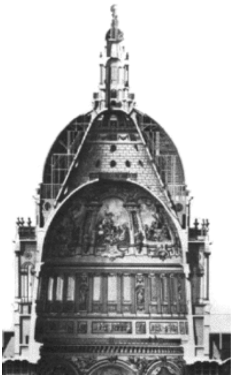
Cross-section showing the brick cone between the inner and outer domes
