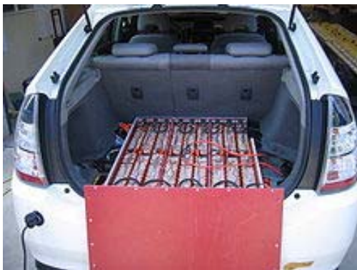
Lithium-ion battery pack, with cover removed, in a CalCars "PRIUS+" plug-in hybrid converted Toyota Prius converted by EnergyCS
