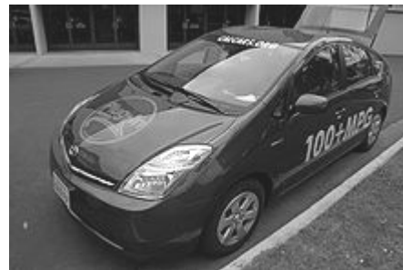
The Toyota Prius converted plug-in hybrid is a series-parallel hybrid
