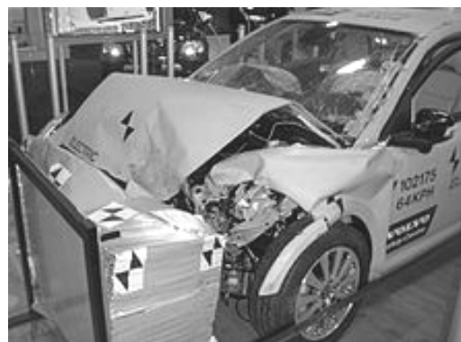
Frontal crash test of a Volvo C30 DRIVE Electric to assess the safety of the battery pack
