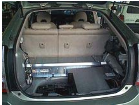
Hybrids Plus plug-in hybrid Toyota Prius conversion with PHEV-30 (30 mile or 48 km all-electric range) battery packs
